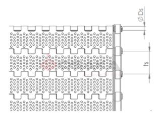
This belt is quite different type comparing with wovens types. This belt producing connections at plates together. It is easy to do washing and drying with this belt because of the holes on the plates. Straigth and wide surface provide to carry heavy loads.
