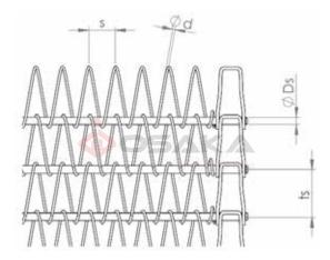
This belt specially used in freezing process which we use these products in daily. The advantage of using this belt to save area in your production because of able to use storeyed and working in - 45 c, Generally raw materials are prefered as spring wire to make more durable belt. Turing factor is 1,60. For example 1040 mm is turning ratio of radius of belt 650 mm width.
