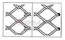
This belt has woven type which seems as decorative belt. It is able to produced with various pitch and wire diameter in copper wire and brass wire. It is useful bothin decorative and conveyor wire belt.
